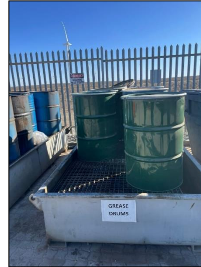
14. Grease drums stored in secondary containment
